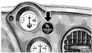
Passenger Airbag Off Light To Shut Off the Passenger Airbag:
